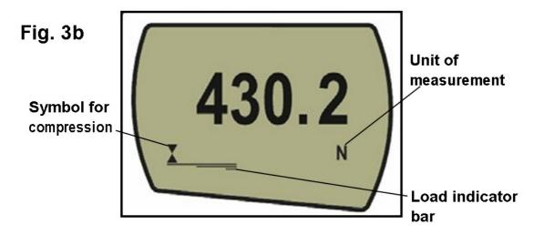
If the AFG has suffered a serious overload condition, the load indicator bar will be partially displayed even when no load is present. This is a warning that the load cell is damaged and you should immediately contact your supplier to arrange repair.
