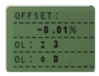
The offset value provides an indication of the condition of the loadcell, and is defined as the % difference between the initial zero and the current zero reading.
