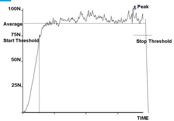
This function allows the average load reading to be displayed. The average starts being calculated when the START threshold (% of full-scale) is reached and stops being calculated when the load passes through the STOP threshold.
