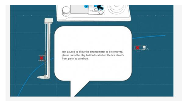
In this example from operation 4 the test runs until 3% strain is reached and pause. At this point the image above is shown, to continue safely remove the extensometer and press the play button located on the front of the test stand.
