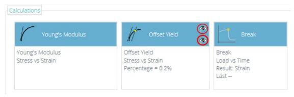
The Offset Yield result that was chosen with **Hide** 'options has two struck-through eye symbols to denote the hidden feature is enabled.
