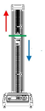
For a compression test, a downwards motion is positive (blue arrow), with upward being negative (red arrow).
