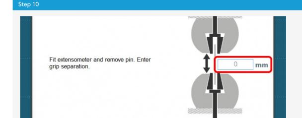
After the pre-load stage, the onscreen pop-up shown in the image above appears. The grip separation should be measured and entered it into the box highlighted above, once ready press the accept button onscreen.
