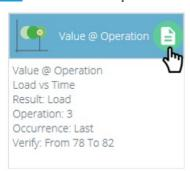
The value at operation result is used to return a specified value at the desired point on the operation timeline. Clicking on the edit button at the top right of the result opens the following window:
