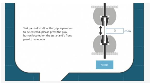
After the pre-load stage, the onscreen pop-up shown in the image above appears. The grip separation should be measured and entered it into the box highlighted above, once ready press the 'Accept' button onscreen.
