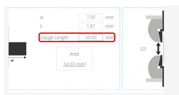
It is important that the initial gauge length of the extensometer device is entered in the **Specimen**' tab of the test designer, as shown in the image above.
