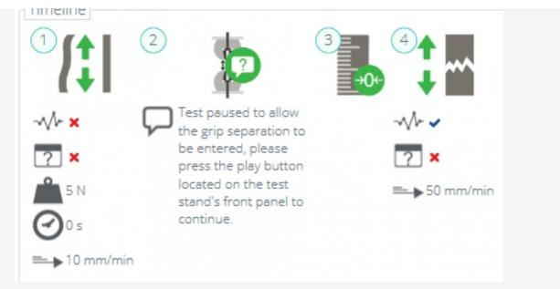
Next, navigate to the **Operations**' tab and configure a suitable preload stage for the test sample, see operation 1 above,
