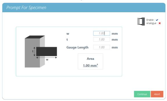
The extensometer settings are displayed in the top right of the prompt for specimen window.
