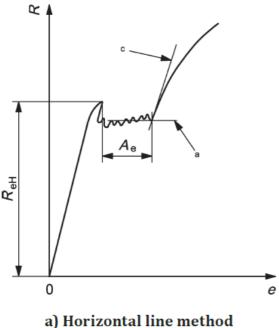
Figure 7 (from ISO-6892-1-2016) — Different evaluation methods for percentage yield point extension, Ae
