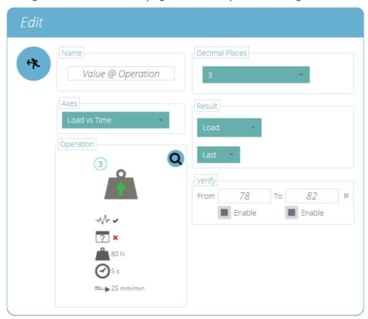
Within this operation, there are two additional important settings. First is the **Operation**' section. Clicking the magnifying glass opens an additional window where the desired operation that the result is to be determined from, can be selected. In the example above operation number 3 has been selected.
