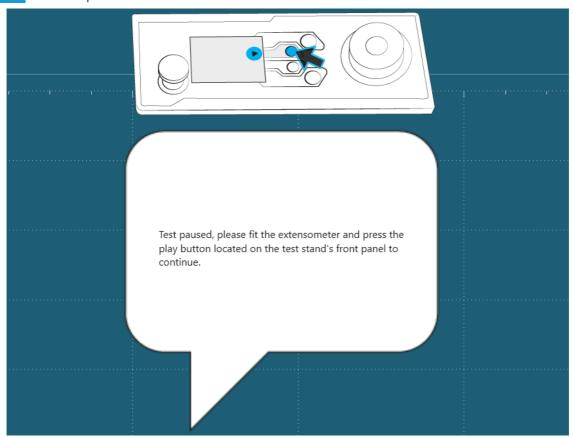
The pause operation in VectorPro stops the test stands movement and display a popup text message when the operation is reached in the test timeline. The text displayed can be set by editing the operation settings in the test timeline. In the example above the message prompts the user to fit an extensometer. To continue the test the user must press the play button on the front panel of the test stand.
