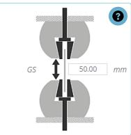
In the example above an extensometer with a gauge length of 50 mm is being used.
