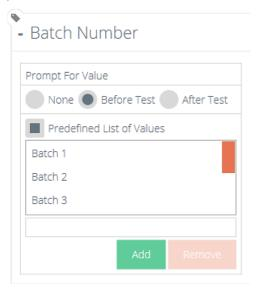
In the example shown both above and below a label attribute called **Batch Number**' is configured within the test designer with '**Before Test**' selected and a predefined list of batch numbers entered.
