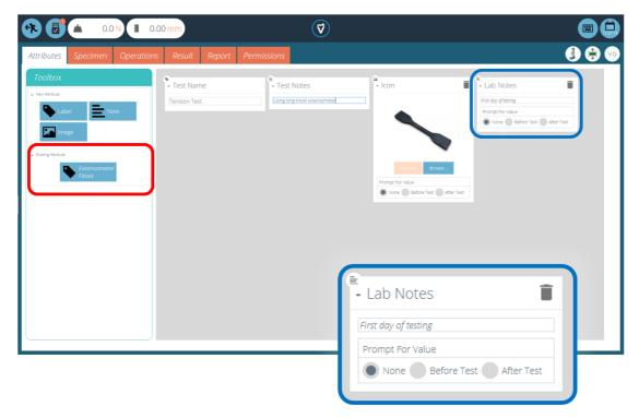
Within the relevant test, place the desired attribute. For example, in the screen above an attribute called **Lab**Notes' is being used by the operator to describe the test being executed. Previously used attributes can be found in the 'Existing Attributes' section (highlighted in red).
