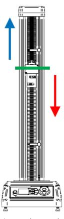
In a tension test, the upward motion is positive (blue arrow), with downward being negative (green arrow).
