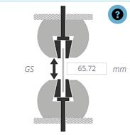
In the example above grip separation is being used to derive strain. The starting separation is 65.72 mm.
