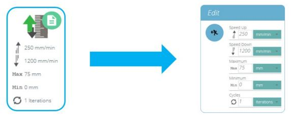
Every operation has parameters that can be edited. Such as displacement, target load, hold time and speed. Below is an example of an operation edit window; this is for a load based drive stage.
