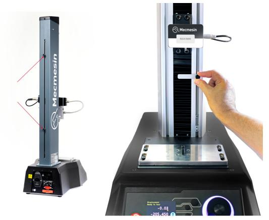
This will stop the crosshead movement at an upper or lower limit during a test sequence. The machine can be driven away from a stop position using the jog controls on the front panel.
