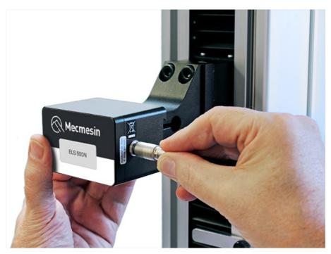
Removal of the load cell connection is made by pulling back the outer body and gently removing the two parts.
