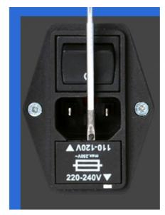
The fuse holder can be ejected using a small flat-blades screwdriver and applying gentle pressure to the upper edge of the fuse holder carriage as indicated below in the right-hand image.
