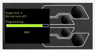
The flashing of the device is carried out automatically and progresses through several stages. It is important that the test stand is not turned off or disconnected. Disconnection of the ELS could lead to irreversible damage.
