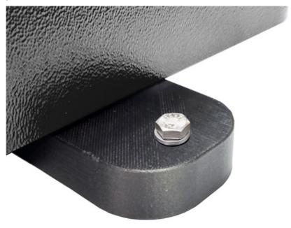
Then, thread the supplied screw through the foot clamp and the work surface. Using the supplied nut and washer secure the foot clamp below the work surface.
