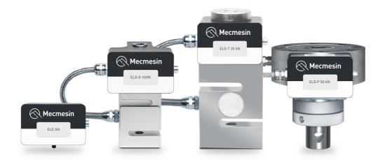
Enhanced load sensors or **ELS**' for short, are smart devices used to capture load readings for the OmniTest test stand. All calibration information is held on the individual load cell making them transferable from system to system and the calibration will follow, with no user input required.
