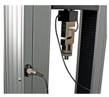
Connecting the ELS to the test stand.
