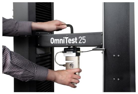
Securing the loadcell with the central M18 holt
