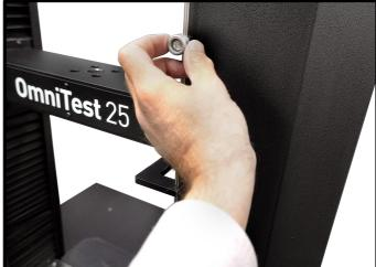
Limit stops on an OmniTest Twin Column
