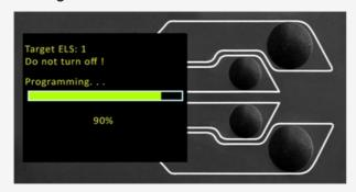
The flashing of the device is carried out automatically and progresses through several stages.
