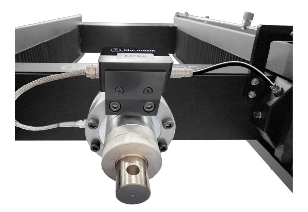
Attach this loadcell to the crosshead using the eight M8x60 socket cap head bolts, using two to locate the loadcell's electronics housing. These screws are 12.9 grade steel with a recommended maximum torque value of 41 N.m. If required the torque values can be checked after first use.
