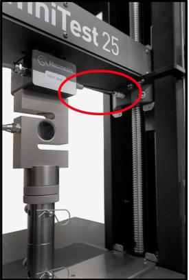
To start the update connect the ELS to the test system, then switch the test stand on.
