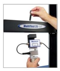
Attaching a loadcell on a twin-column system
