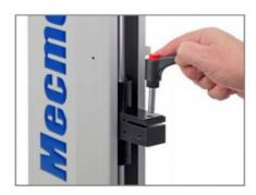
Inserting the adjustable handle lever
