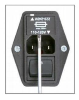
Fuse carrier / Carrier removal
