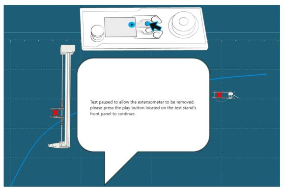
This operation allows the extensometer to be removed during the test, before a break condition. This is crucial if the elongation range of the specimen is higher than the device's measurement range, for a test method requirement, or for the preservation of extensometers when high energy break test specimens are measured.
