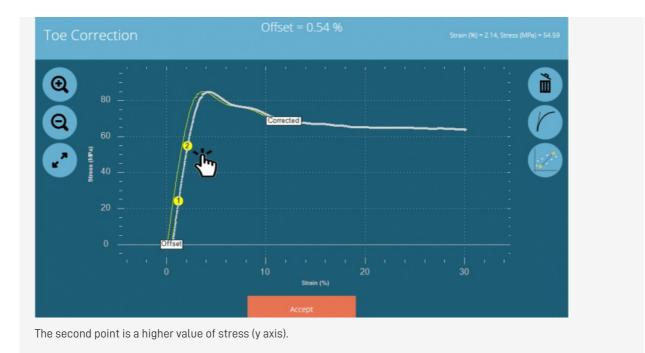
Once the second point (higher value of stress), the display will automatically switch to show the manually calculated screen, which contans the following information or functions:
