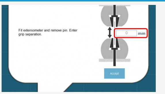
After the pre-load stage, the onscreen pop-up shown in the image above appears. The grip separation should be measured and entered it into the box highlighted above, once ready press the accept button onscreen.
