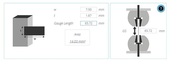
In the example above grip separation is being used to derive strain. The starting separation is 65.72 mm.
