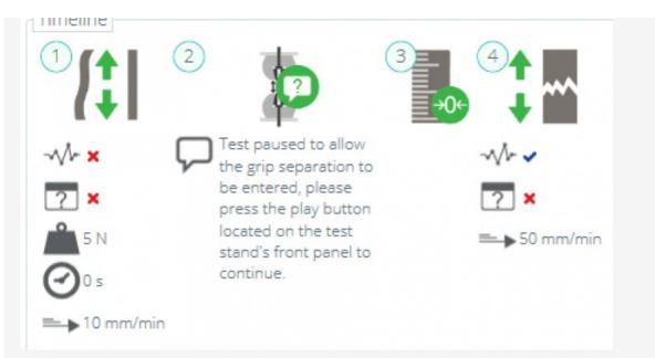
Next, navigate to the 'Operations' tab and configure a suitable preload stage for the test sample, see operation 1 above,
