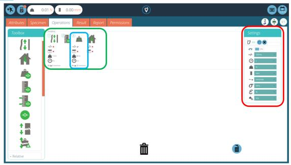
The 'Timeline' is where drag-and-drop operation commands from the left-hand **Toolbox**' are placed. This defines the test running sequence. In this instance the user has chosen to run a test that consists of:
