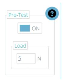
Pre-test preload allows the application of a specified force to the specimen prior to commencing the main operation sequence.
