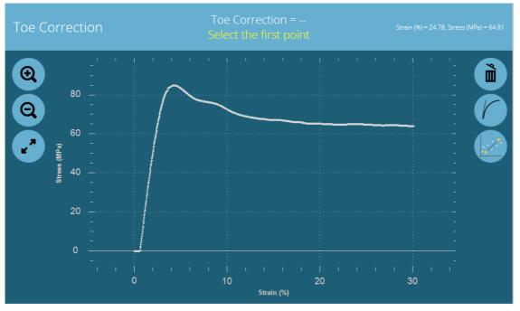
The user will be requested to select two points for which a cord line will be drawn between. This will determine a slope and ultimately the toe correction offset value and line which intercepts the strain axis.
