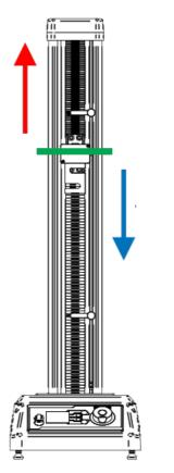
For a compression test, a downwards motion is positive (blue arrow), with upward being negative (red arrow).
