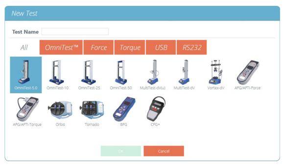
The 'New Test' selection screen, select which instrument is used.
