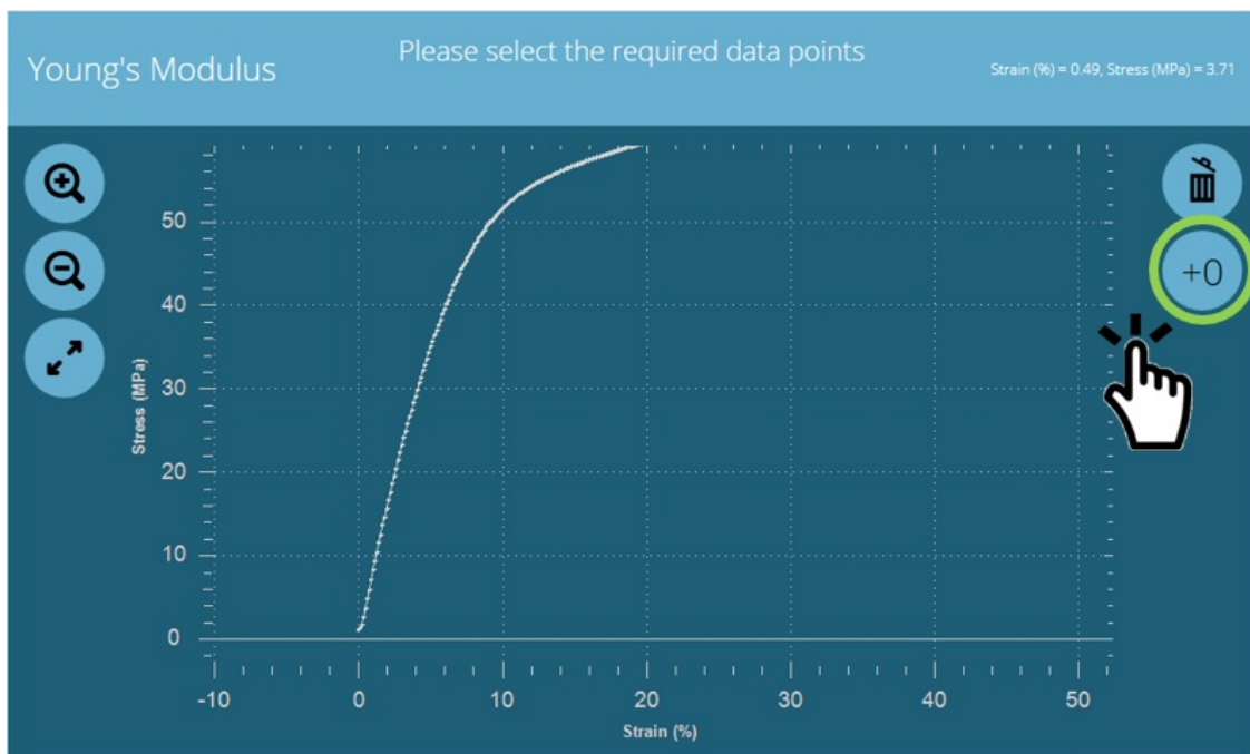
An example of a secant modulus selected.
