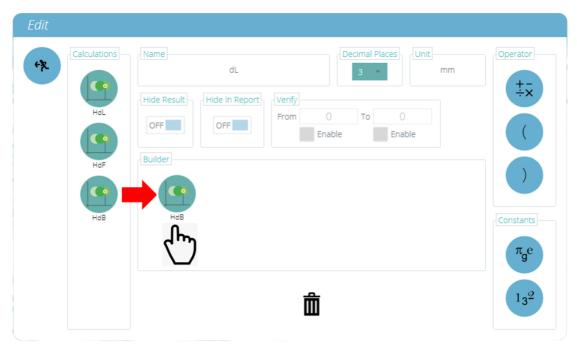
To configure an operator/constant, place the desired component into the formula builder, then click on the component to reveal the operator or constant settings menu. As shown in the image below:
