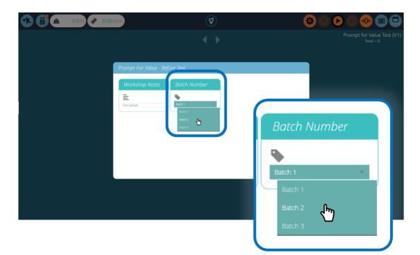
Upon starting the test, the **'Prompt for Value – Before Test**' window appears. Entry input is available, for any attributes that have been configured to prompt before the test is run.
