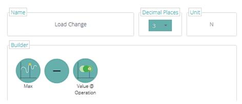
In the image above the load change for the test is being calculated by subtracting the result of the **Value @ Operation**' calculation from the result of the 'Max' calculation.
