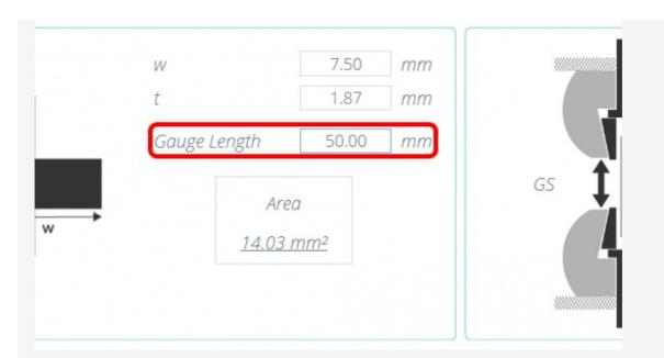
It is important that the initial gauge length of the extensometer device is entered in the **Specimen** tab of the test designer, as shown in the image above.
