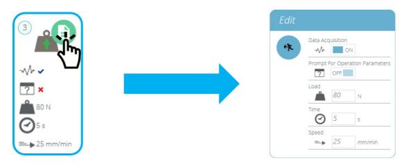
Each operation has parameters that can be edited. Such as displacement, target load, hold time and speed. Below is an example of an operation edit window; this is for a load based drive stage.
