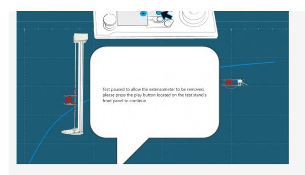
In this example from operation 4 the test runs until 3% strain is reached and pause. At this point the image above is shown, to continue safely remove the extensioneter and press the play button located on the front of the test stand.
