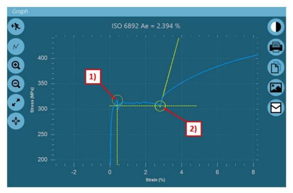
Should the user select the user-defined range option, this will invoke a user input screen that requires manual selection of data points using a mouse or touch screen cursor.
