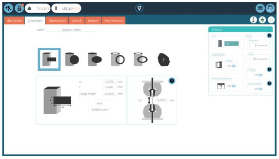
The "**Specimen**' screen is used to define physical dimensions of the specimen, configure the extensometer and configure break settings.
