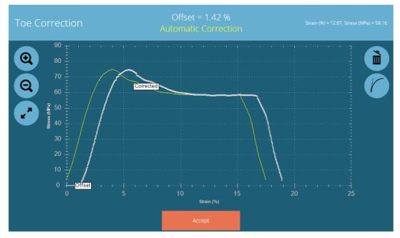
When the test sequence has ended, the screen above will be shown for **Automatic Correction**' and contain s the following information or functions:
