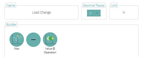
In the image above the load change for the test is being calculated by subtracting the result of the **Value @ Operation**' calculation from the result of the 'Max' calculation.
