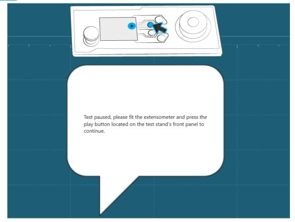
The pause operation in VectorPro stops the test stands movement and display a popup text message when the operation is reached in the test timeline. The text displayed can be set by editing the operation settings in the test timeline. In the example above the message prompts the user to fit an extensometer. To continue the test the user must press the play button on the front panel of the test stand.
