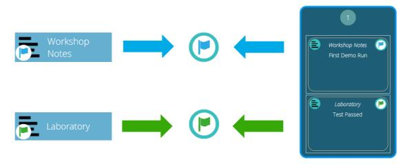
A diagram displaying the new flag markers. The left-hand icons are the markers within the**Results**' design page and the right hand are within the '**Results Viewer**'. Before test flags are highlighted in blue and after test flags are highlighted in green.
