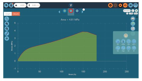
When selecting the calculation all other samples are hidden and a visual overlay is added to the display where the calculation is taking place. This can be saved for export using the graph capture buttons.
