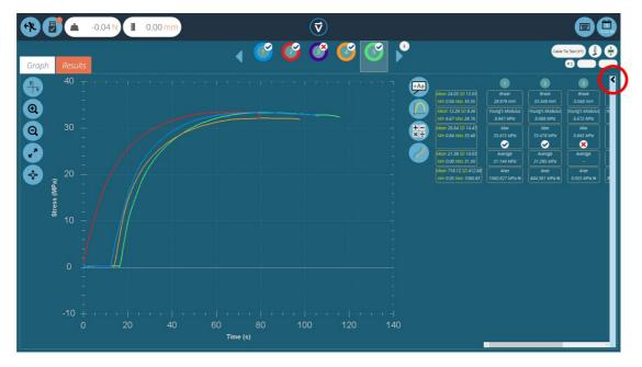
Additional spot calculations can be used by clicking the **Apply spot calculation**' icon. The selected calculation will apply to the currently selected sample and its current viewable X-Y range.
