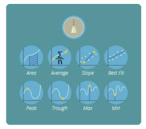
Within this menu there are two main functions; the broom icon, this deletes any currently applied calculation and the calculation section. Here the user can select the desired calculation to apply to the currently selected sample.
