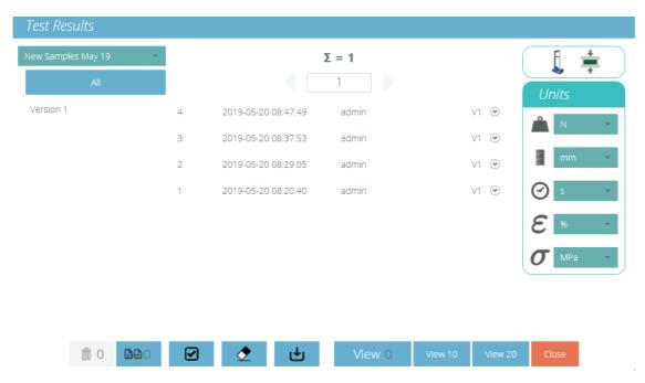
Here, four results from the test have been selected. The results display can be filtered their number on the left-hand side of the screen. In the image above 'All' versions have been selected. To view the tests simply click View'. Options to select 'View 10' and View 20' to open a predefined number of tests are available. When using the Results' viewer be aware that:
