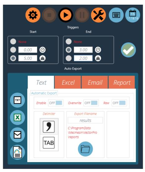
In the image above pressing play will start the test operation, data capture will begin once the indicated load is above 5.00N. Data capture will stop once the time elapsed has reached 3.00 minutes.
