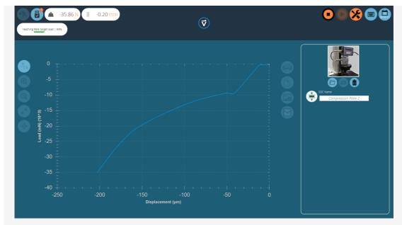
The test will now begin, the initial two stages (pre-load phase and 90% run) are not captured. Test status is indicated by the progress bar located in the upper left corner (pictured above).
