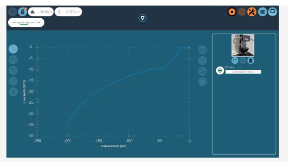
The test will now begin, the initial two stages (pre-load phase and 90% run) are not captured. Test status is indicated by the progress bar located in the upper left corner (pictured above).
