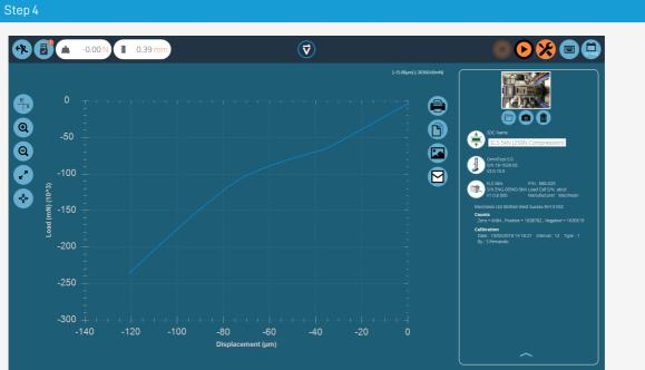
During the final 95% run the data will be captured, the image below shows a curve for an Omnitest-5 being run in compression. Values are captured in mN and  $\mu m.$
