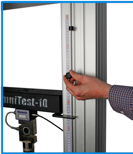
Limit stops on an OmniTest twin column
