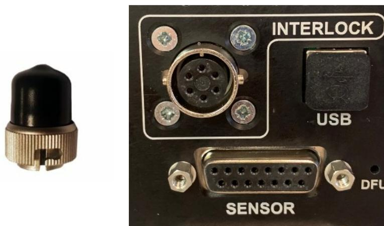
Interlock override plug (351-102) and Interlock rear panel connection on a Mark 2 Interlock enabled MultiTest-*dV*
