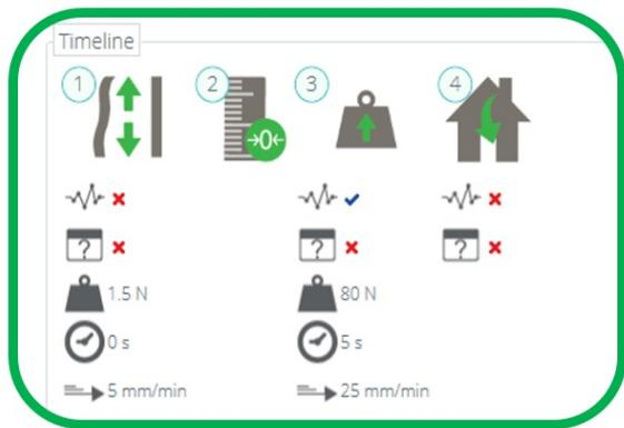
1. Preload Specimen (to a force of 1.5N at 5mm/min) →
