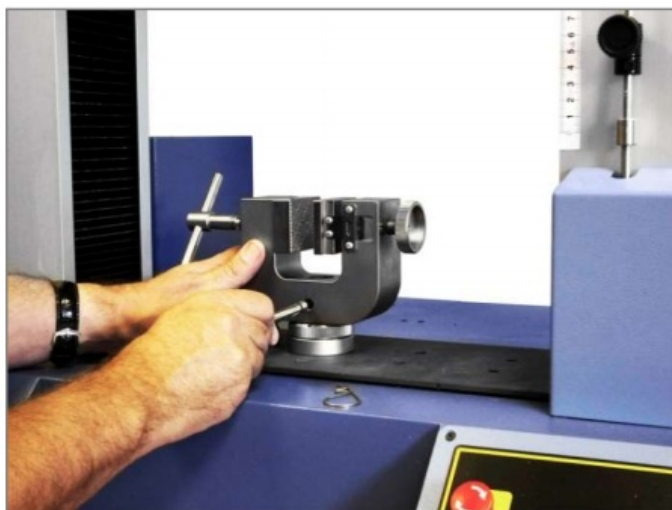
Attaching a grip with the QC quick interchange fittings
