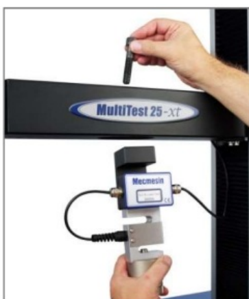
Attaching a loadcell on a twin-column system
