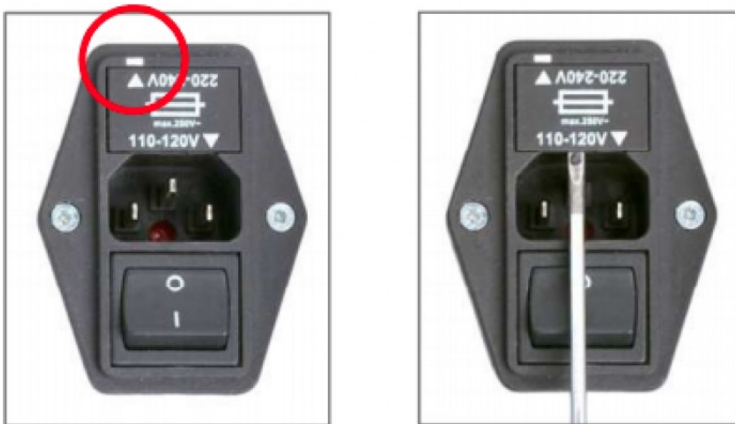
Fuse carrier / Carrier removal
