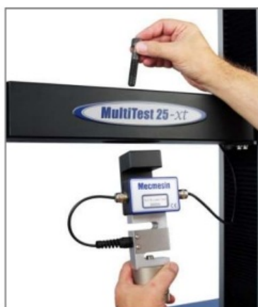
Attaching a loadcell on a twin-column system
