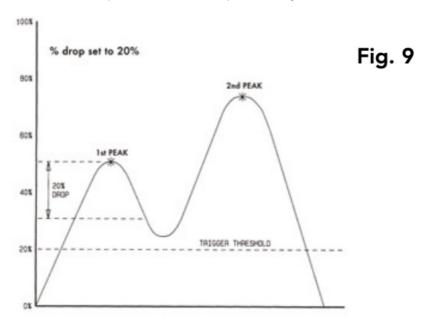
To enable the % 1st PEAK function, press and hold the MENU key until page 1 of the main menu appears. Press the DOWN key to move the cursor to % 1ST PEAK and press the ENTER key.
