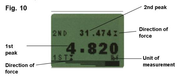
When setting up the Force Gauge, a graphical representation of the test provides a clear insight into the % drop factor required. Please contact James Heal or your approved supplier for details on Dataplot graphical charting software.
