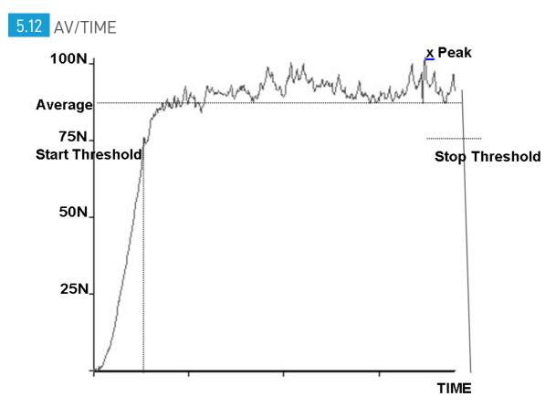
This function allows the average load reading to be displayed. The average starts being calculated when the START threshold (% of full-scale) is reached and stops being calculated when the load passes through the STOP threshold.
