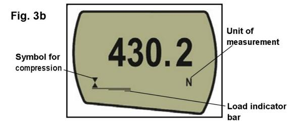
If the Force Gauge has suffered a serious overload condition, the load indicator bar will be partially displayed even when no load is present. This is a warning that the load cell is damaged and you should immediately contact your supplier to arrange repair.
