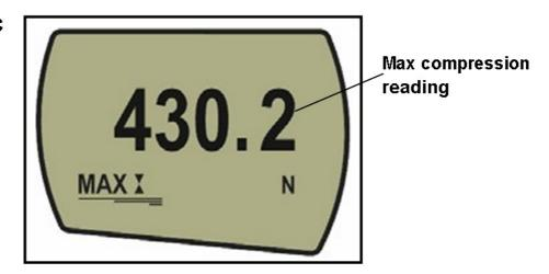
Note: When % 1st PEAK function is enabled, different max modes are shown
