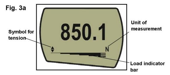
A load indicator bar alerts the operator to how much load has been applied to the loadcell. As the load approaches the maximum rating of the loadcell, the indicator bar changes appearance when above approximately 80% of the rated capacity. This warns the operator that steps should be taken to prevent excessive load being applied.
