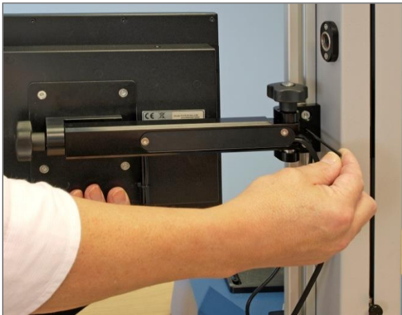
Using the Allen (hex) key, adjust the console height
