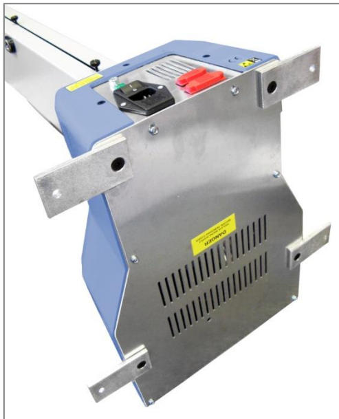
MultiTest 0.5-xt and 1-xt are supplied with anchoring brackets
