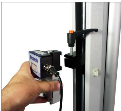
Slide the loadcell onto the dovetail ...
