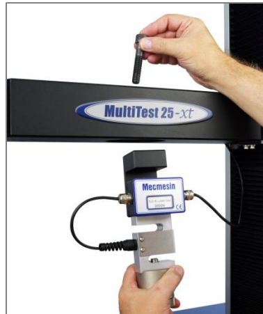
Attaching a loadcell on a twin-column system
