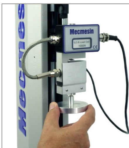
ILC-S and compression plate fitted to a MultiTest 1- xt
