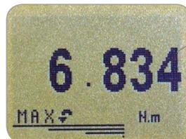
Max counter-clockwise reading
