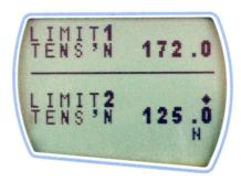
Note: The alarm limits are not active below 1% of the capacity of the tester.
