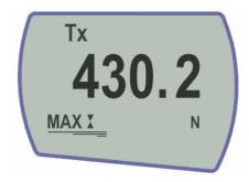
To stop sending data, simply press and release the TXD key, at which point TX will disappear from the display.
