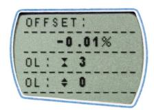
The offset value provides an indication of the condition of the loadcell, and is defined as the % difference between the initial zero and the current zero reading.
