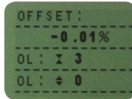
The offset value provides an indication of the condition of the loadcell, and is defined as the % difference between the initial zero and the current zero reading.
