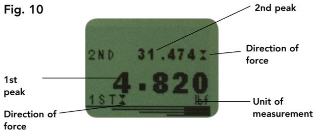
Example: AFG 100N has % drop of 20 (= 20N). If the peak load before sample break is 50N, the load must drop to 30N in order for the AFG to detect a 1st peak of 50N. If load continues to be applied above 50N (e.g. to 75N), the AFG will return 75N as MAX and 50N as 1st peak.
