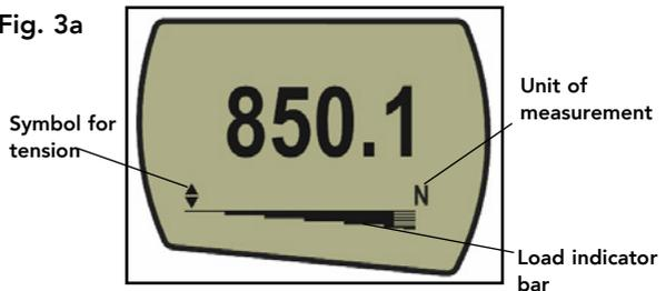
A load indicator bar alerts the operator to how much load has been applied to the loadcell. As the load approaches the maximum rating of the loadcell, the indicator bar changes appearance when above approximately 80% of the rated capacity. This warns the operator that steps should be taken to prevent excessive load being applied.
