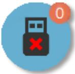
The 'USB' icon, located at the top left of your VectorPro software shows what devices are connected. When showing a tick, this indicates that a test system is connected and switched on. When a system is not active (and for serial instruments on their own), the tick is replaced by a red cross.
