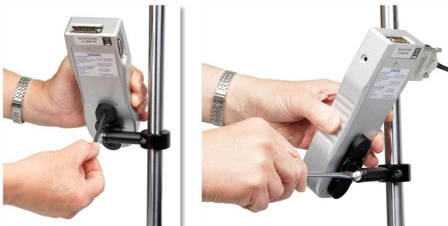
▲ The left-hand image shows the AFTI being secured to the bracket, while the image on the right shows how to adjust the angle of the AFTI.
