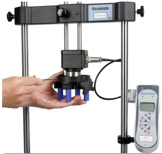
The most commonly-used lower fixture is the 188 mm diameter lower fixing plate with a diameter capacity of 10 mm to 190 mm. This is fixed to the Vortex-*dV* spindle using a 2.5 mm Allen key to secure the four countersunk screws supplied.
