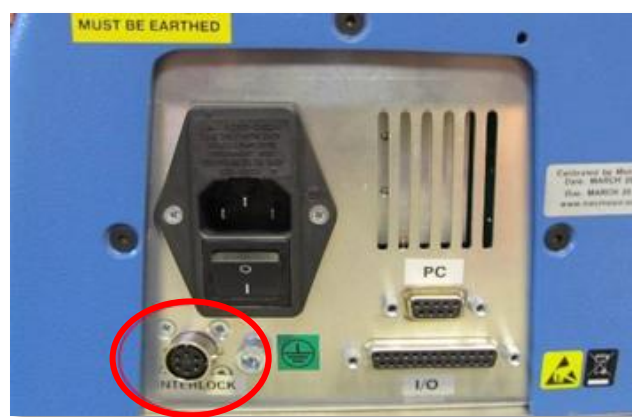
▲ Single Column Interlock Connection
