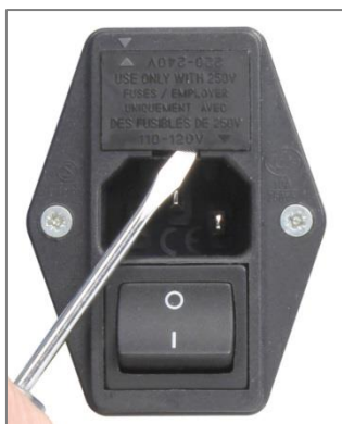
Removing the fuse carrier
