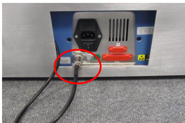
▲ Interlock Guard Cable Connected on MultiTest Single Column
