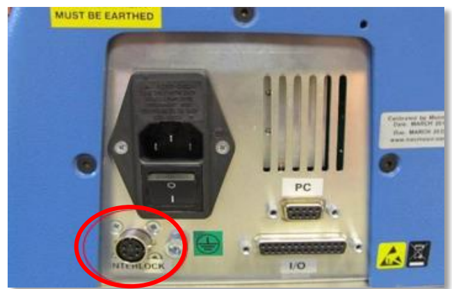
▲ Rear Panel Interlock Connection
