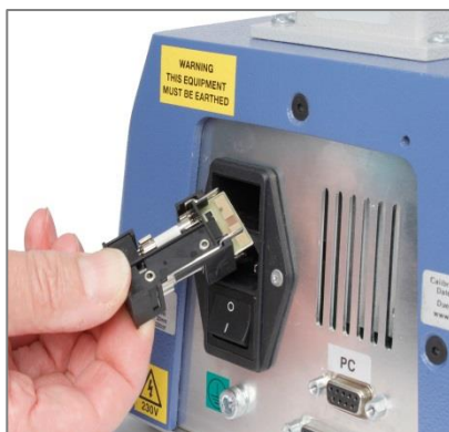
Carrier removed to replace fuse
