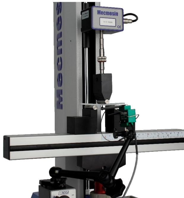
▲ A MultiTest-*dV* 2.5kN in *dV(u)* mode performing a 3-point bend, using an ELS 500N and deflectometer
