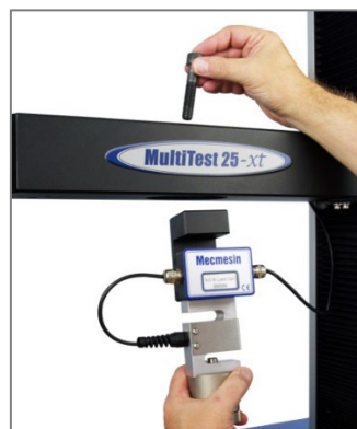
Attaching a loadcell on a twin-column system
