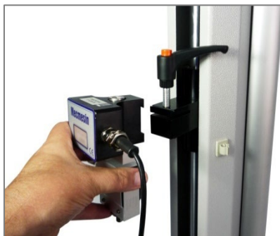
Slide the loadcell onto the dovetail ...
