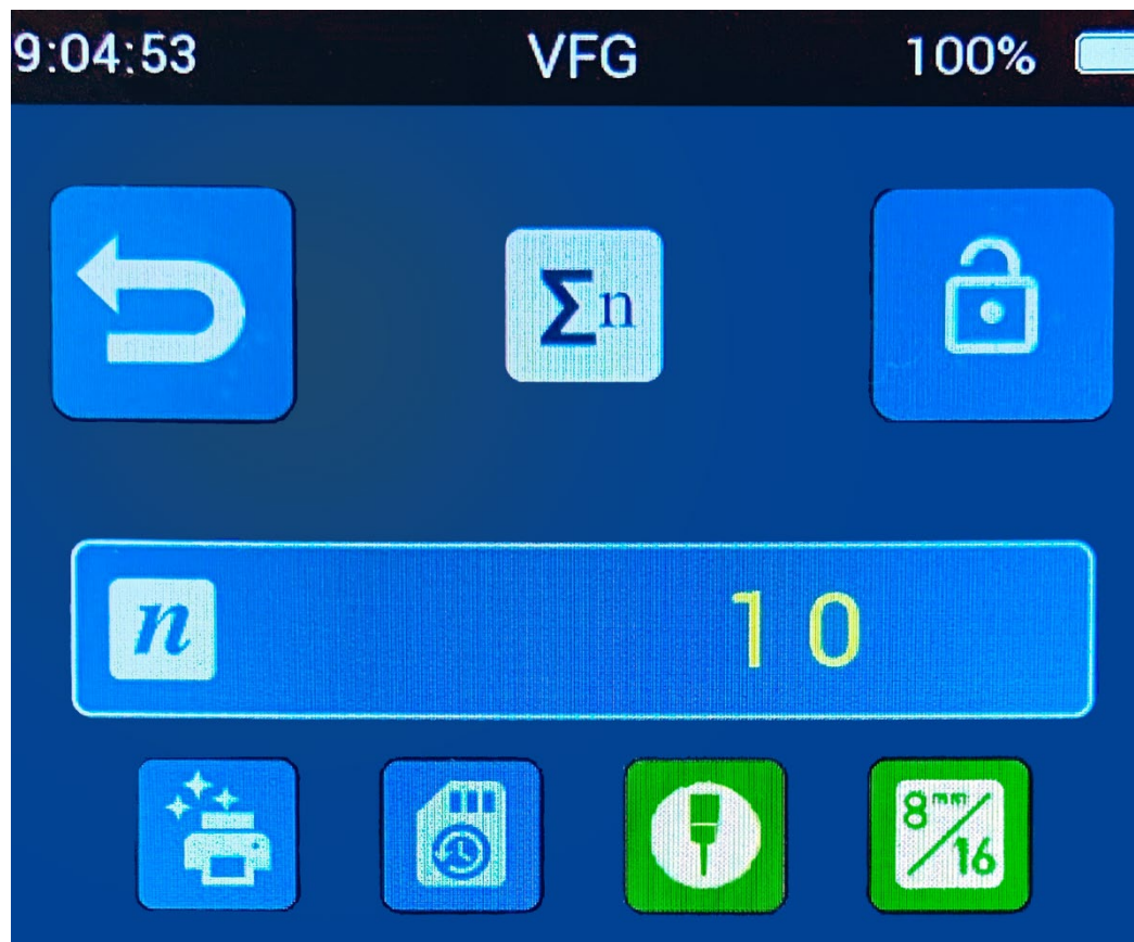
Statistics settings to perform shotcrete strength calculations (with 8 mm aggregate option)
