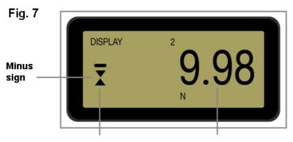
Symbol for compression Max compression reading
