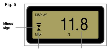
Symbol for compression Max compression reading
