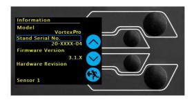
This screen is used to display vital information relating to your VortexPro and the connected ETS sensor including software, hardware, and firmware properties. You can also review calibration data for the test system.
