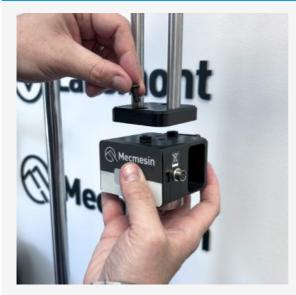
Align the torque sensor with the mounting plate and secure using the two 4 mm Hex screws.
