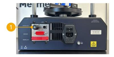
Mecmesin interlocked guarding is fitted with a cable and plug from the guard, that must be fitted to the rear of the stand panel 'Interlock' connection, in place of the removed override plug.
