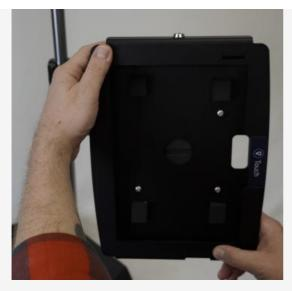
Ensure the console holder front plate is unlocked using the key. Attach it to the back plate and then lock the front plate to secure your console. Adjust the angle of the arm and the orientation of the console as needed. Finally, tighten each hex screw on the support arm joints and ball-joint to secure the desired position.
