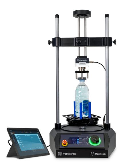
VortexPro automated torque tester, powered by VectorPro
