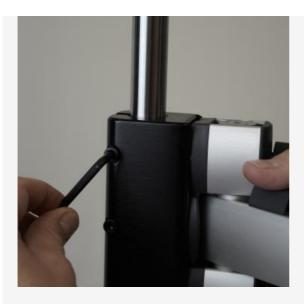
VortexPro - Tighten screws in console column bracket
