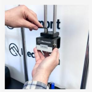
If needed, have one person hold the sensor while the other fits the screws. Ensure the sensor is seated centrally before tightening the screws.
