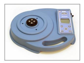
Step 2: Align top plate with torque drive. The handle is positioned to the left.
