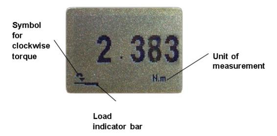
A torque indicator bar alerts the operator to how much load has been applied to the torque sensor. As the load approaches the
