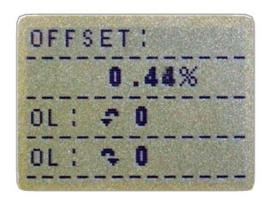
The offset value provides an indication of the condition of the torque sensor, and is defined as the % difference between the critical zero and the current reading.
