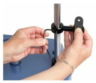
To fit the AFTI to the bracket use the two supplied screws. These pass through the bracket into the back of the gauge and are secured using a 4mm Hex key. The angle the AFTI sits at can be adjusted by loosening the screw located on the side of the bracket.
