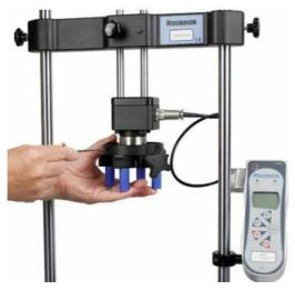
The most commonly-used lower fixture is the 188 mm diameter lower fixing plate with a diameter capacity of 10 mm to 190 mm. This is fixed to the Vortex-dV spindle using a 2.5 mm Hex key to secure the four countersunk screws supplied.
