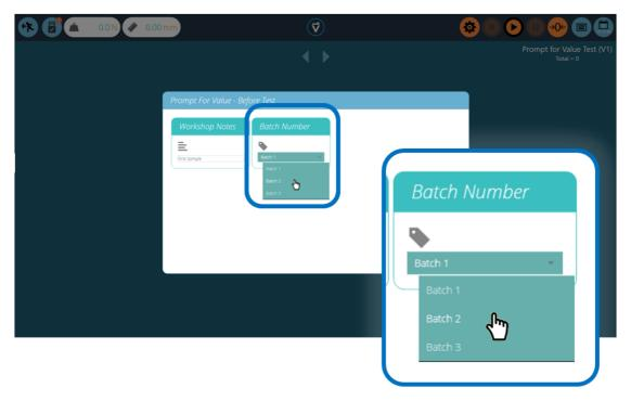
Upon starting the test, the **Prompt for Value – Before Test**' window appears. Entry input is available, for any attributes that have been configured to prompt before the test is run.
