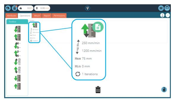
The 'Timeline' allows drag-and-drop of the selected operation command from the left-hand Toolbox' to define the test function. In this instance the user has chosen to run a test that consists of:
