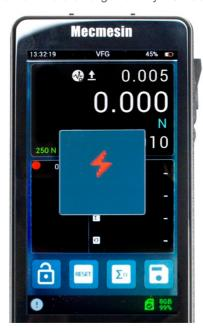
Your Vector Instrument uses a relatively high power battery. This means that it needs a high power charger to provide the instrument with a net popsitive charge. If the power supply you plug into is not designated "PD" then the instrument will show you the popup to tell you that there is not enough power in the supply to charge your device. Just touch the popup to clear it.
