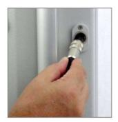
Slide loadcell onto dovetail ... tighten securely ... connect the loadcell
