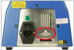
Rear panels of a Vortex-i (left) and MultiTest-i (right). Plug the USB cable into the circled PC socket.
