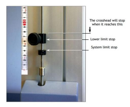
Lower limit stop and system limit stop on a twin-column stand, upper and lower limit stops
