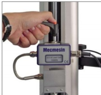
Slide loadcell onto dovetail ... tighten securely ... connect the loadcell
