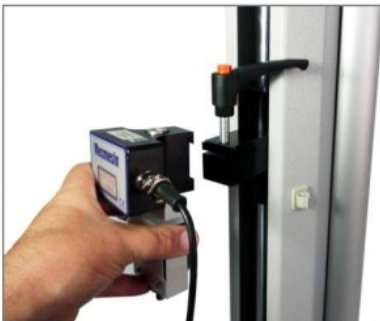
Slide loadcell onto dovetail ... tighten securely ... connect the loadcell
