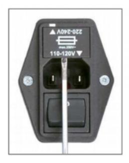
Fuse carrier / Carrier removal
