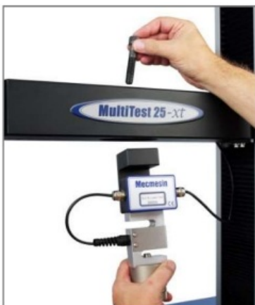
Attaching a loadcell on a twin-column system
