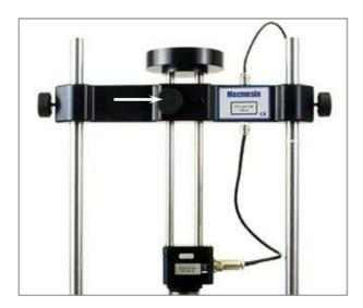
If a top-load is to be used, the securing knob (arrowed) is generally left undone during measurement so the carrier can slide up and down. If a top load is not to be used, securely tighten the locking knob after adjusting to the height required.
