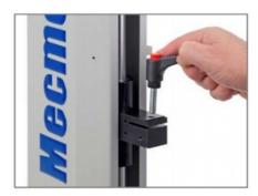
Inserting the adjustable handle lever
