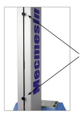
Limit stops on a MultiTest-i. Stops on other stands all operate in the same way.
