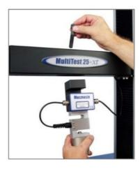
Attaching a loadcell on a twin-column system
