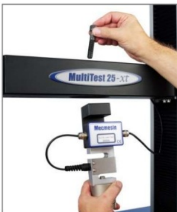
Attaching a loadcell on a twin-column system
