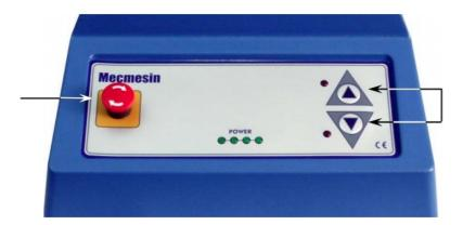
The front panel of the MultiTest 1-i: Emergency stop (left), Jog buttons (right). Vortex-i has a similar emergency stop button and clockwise and anticlockwise jog buttons.
